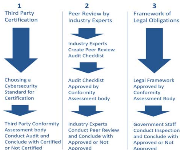
Figure 2: Three tracks to demonstrate the implementation of minimum and advanced cybersecurity requirements of the common electricity cybersecurity framework.
